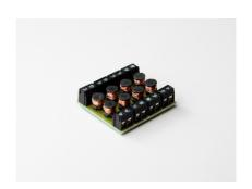
The ACT 2468 RFI Filter is designed to attenuate RFI signals picked up by alarm cables acting as aerials. It snaps apart to make any combination of 2, 4, 6 or 8 wire RFI filters which can be fitted to either or both ends of the alarm circuit cable.
